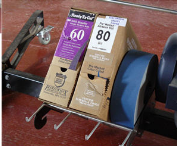
Photo 8. The "Rack 'N Roll" accessory provides convenient under the table storage for sandpaper rolls.
