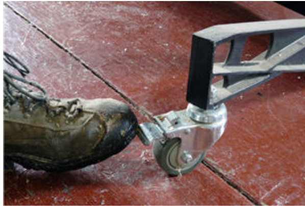
Photo 6. A set of casters mobilizes the sander for easy storage and locks tight to provide a stable platform.
