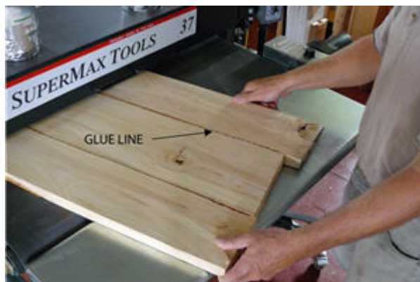
Photo 4. No more scraping glue and tearing wood. 36-grit paper, a skewed feed angle and light passes grinds off the glue globs.
