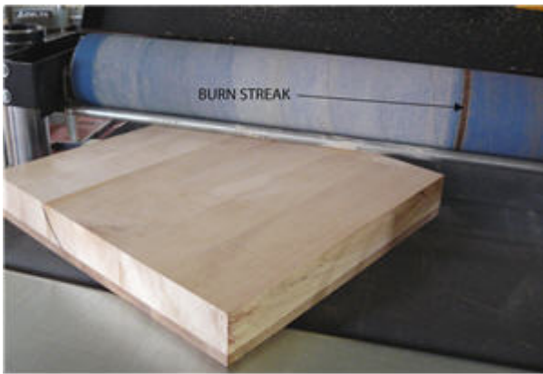
Photo 3. Even with a burn streak on the paper, the wide drum has enough left over capacity to sand most objects without having to trash the whole belt.
