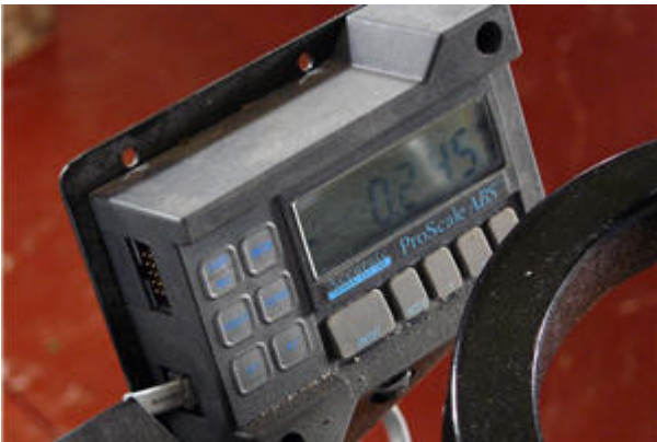
Photo 9. The ProScale linear digital measuring system gives you accurate readings to 1/1000-in. If you ever have to duplicate a piece to an exact dimension, this can be a real lifesaver.
