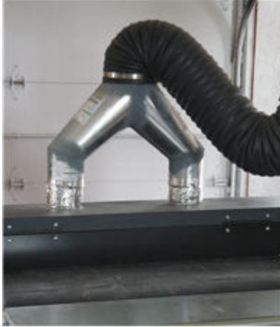
Photo 5. I recommend having a "pant leg" fitting made for the dust collection hood. You can also fabricate your own with a wye fitting and 45-degree elbows to connect to the two 4-inch ports.
