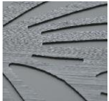
This cut was sanded using a drum or wide-belt sander.
